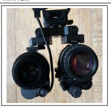
Step 2: Remove the Mini rail on the MH25. Also remove the upper dove tail from the Lower portion of the Dove tail adaptor (DTA). This is in preparation to mount the lower portion of the DTA directly to the MH25. Align the bottom part of the DTA with the housing of the MH25. You will notice the holes in the DTA align perfectly with the holes in the housing.
